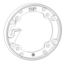
Step 4 Hang the integrated camera into the base along the guide slots and rotate it to a certain angle for facilitate cable connection, as shown in Figure 3-10.
